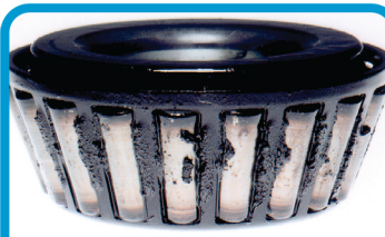
Heavy deposits reduce equipment life.
