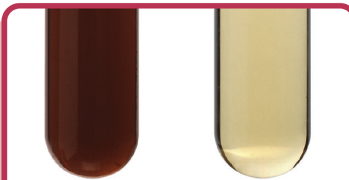
Brake fluid before (left) and after (right) service.
